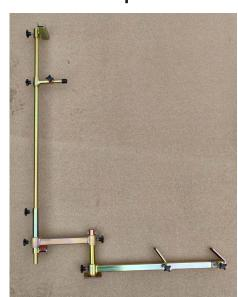
The 'Top Vent Angle' is normally used when the Top Hung Drop Set is fitted, as shown here in the middle of the horizontal arm.
